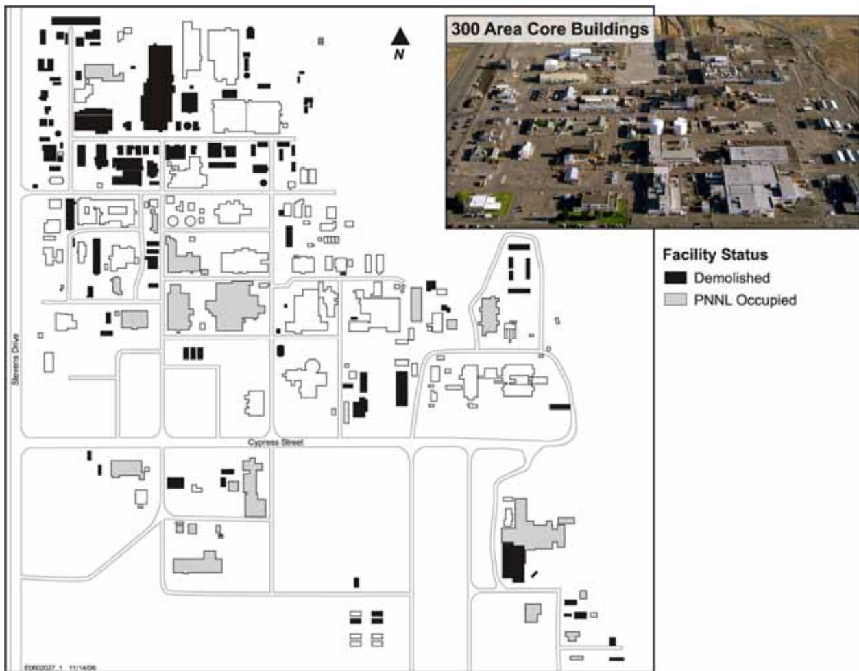
Fig. 1. At the end of CY2006, nearly all of the structures in the northern half of Hanford's 300 Area had been demolished.
