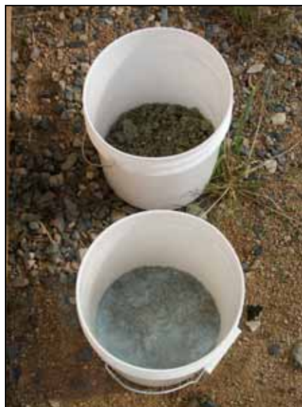
Fig. 2. Proximity chemical reactivity test of solidified nitric acid (lower bucket) and solidified ammonium hydroxide (upper bucket) showing fumes produced from acid bucket.
