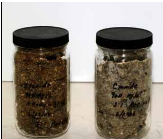
Fig. 4. An oxidized sample of solidified cyanide solution (left) and an unoxidized sample of solidified cyanide solution (right) from the first sample group.
