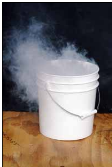
Fig. 3. Contact chemical reactivity test of solidified nitric acid and solidified ammonium hydroxide showing fumes produced due to contact of wasteforms.
