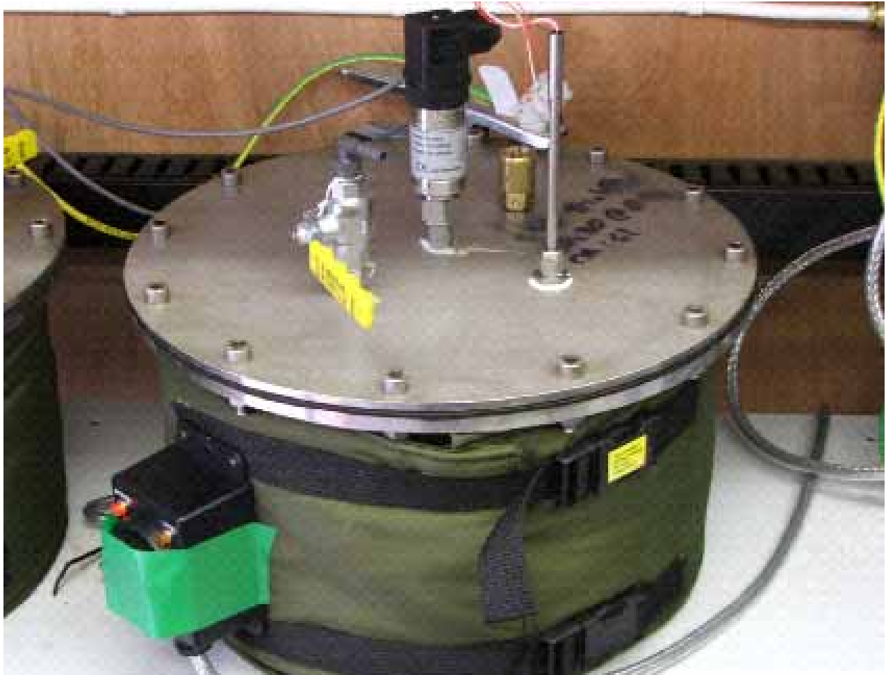
Fig. 1. Stainless steel reaction vessel with pressure transducer, thermometer & heating jacket
