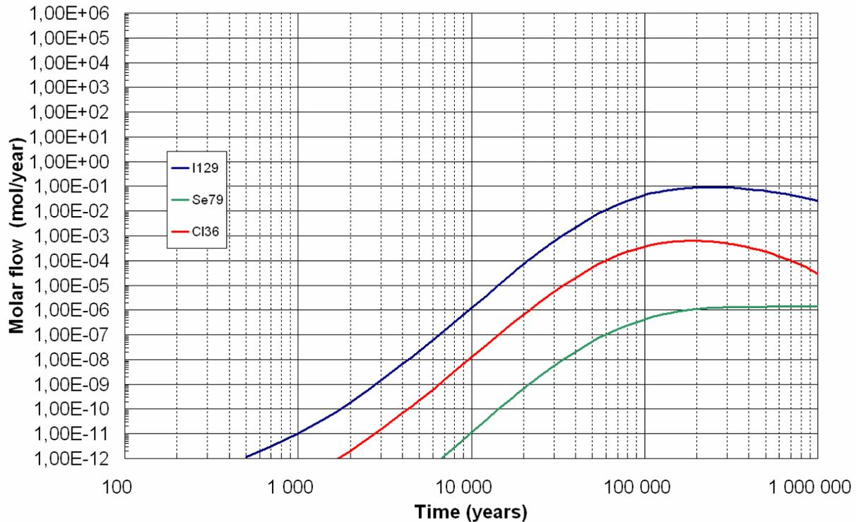
Fig. 3. Molar flow rate of I-129, Se-79 and Cl-36 out of the Callovo-Oxfordian formation.
