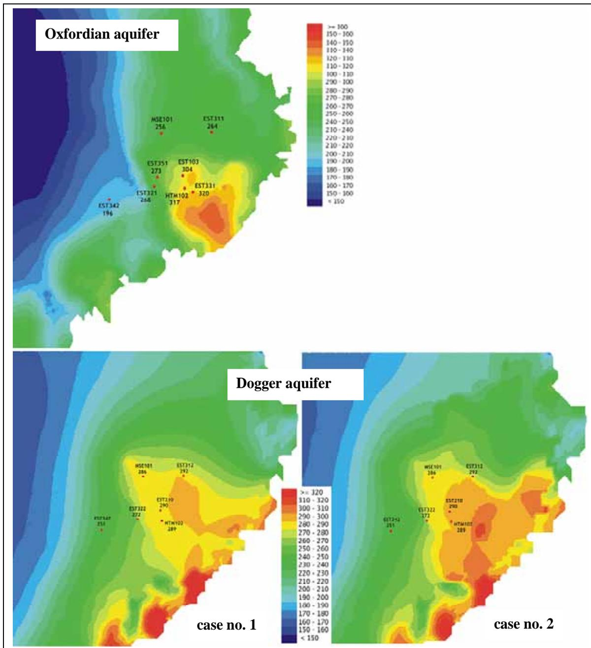
Fig. 1. Computed head values (colors) and measured head values (red dots) for the Oxfordian and the Bathonian aquifer, in case no. 1 and case no. 2.
