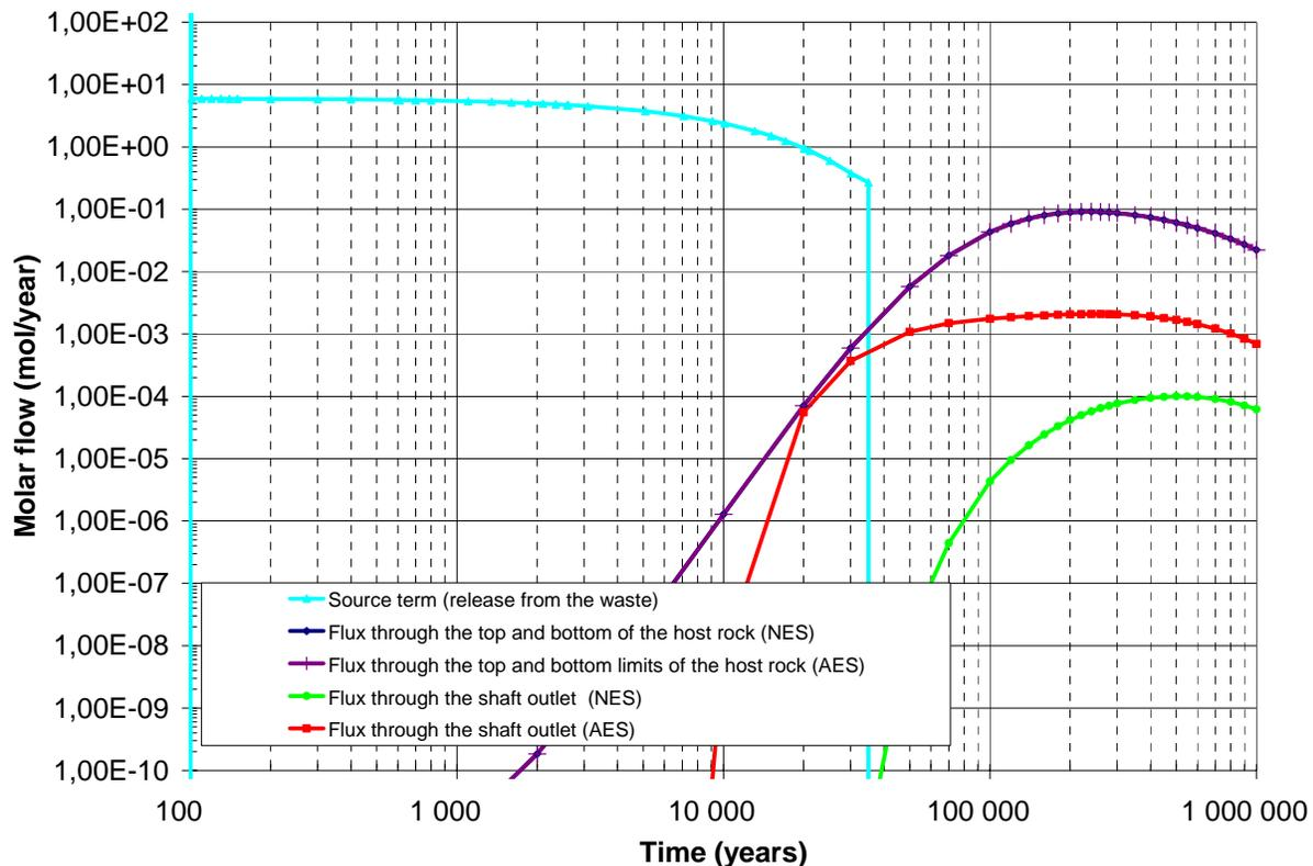
Fig. 2. Molar flow rate of I-129 out of a shaft and the Callovo-Oxfordian formation.
