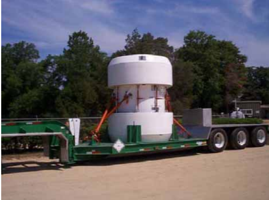
Fig. 1. CNS 10-160B transportation cask
