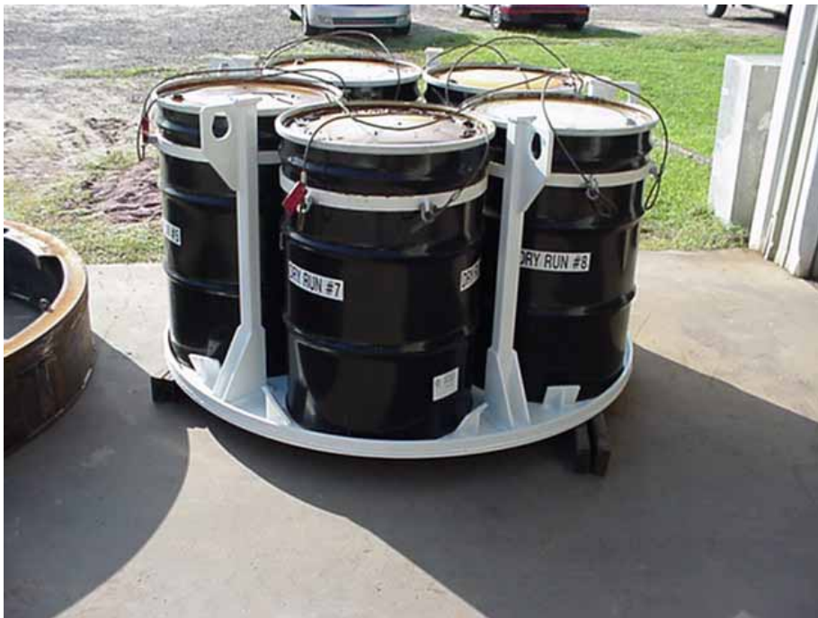
Fig. 2. Arrangement of a 5-pack of drums for placement in the CNS 10-160B cask.
