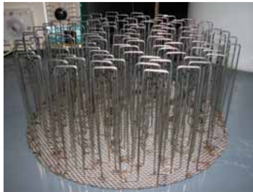
Fig. 2. Model cooling coils placed in the 1-ft diameter tank to mimic HLW type III tanks at SRS
