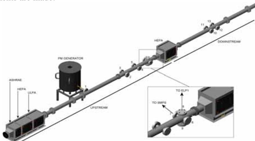
Fig. 1. The ICET HEPA filter test stand and aerosol generator.
