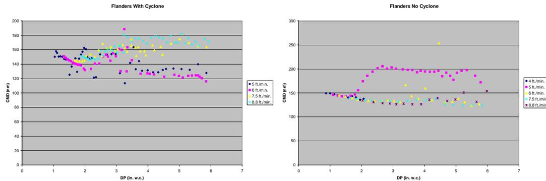
**Fig. 2. Downstream CMD vs. DP for Flanders filters, loading with and without the 3  $\mu\text{m}$  cut-point cyclone in place.**
