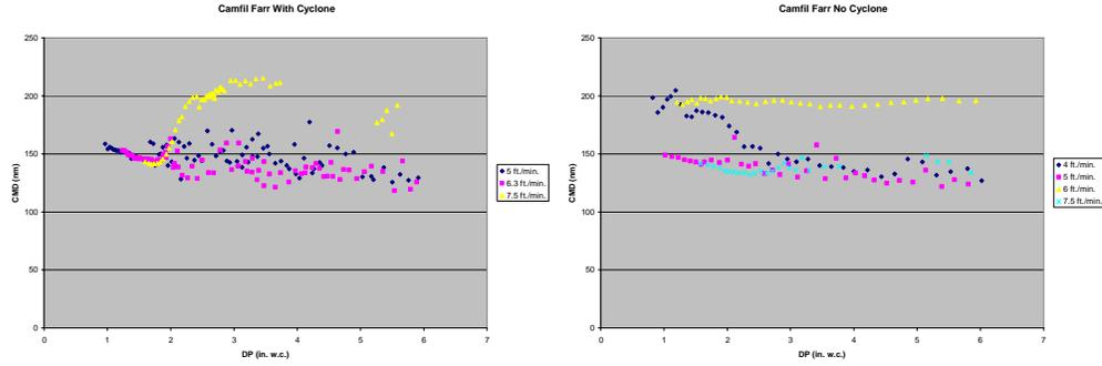
**Fig. 3. Downstream CMD vs. DP for Camfil Farr filters, loading with and without the 3 µm cut-point cyclone in place.**
