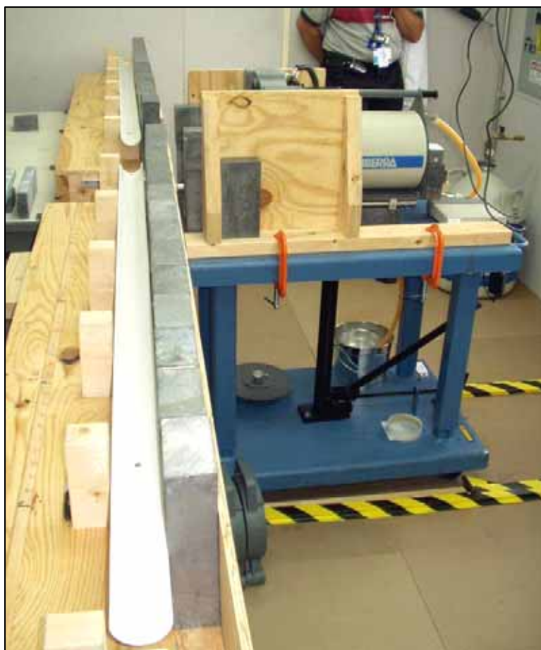
Fig. 1 Photo of one of the high-resolution gamma spectroscopy stations in a trailer at the Corehole 8 Tank W-1A site.
