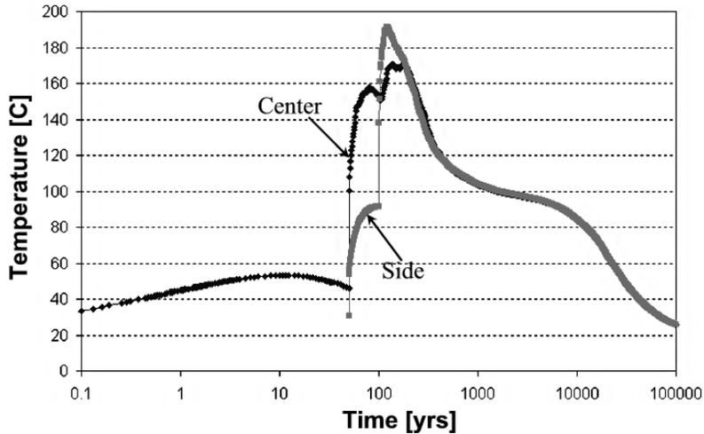
(b) Waste package temperature vs. time for Case 4.
