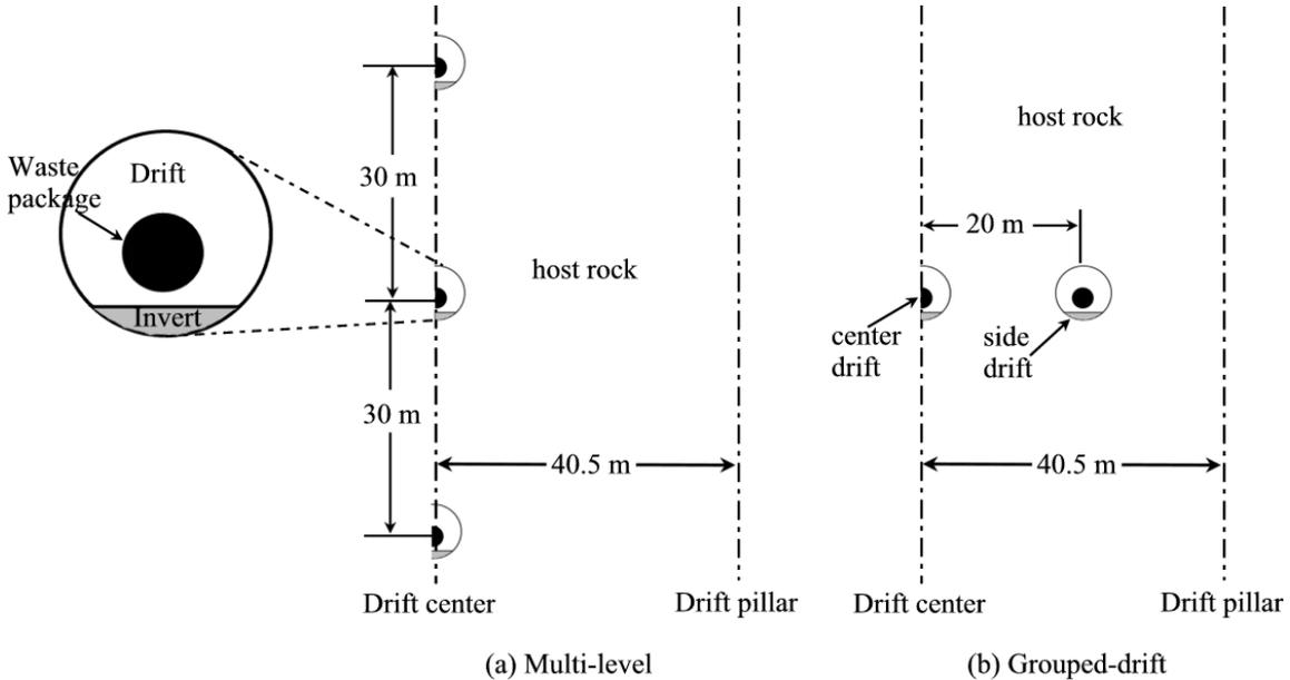
**Fig. 1. Illustration of alternative repository designs for studying spent-fuel disposal capacity in Yucca Mountain: (a) multi-level repository design and (b) grouped-drift repository design.**
