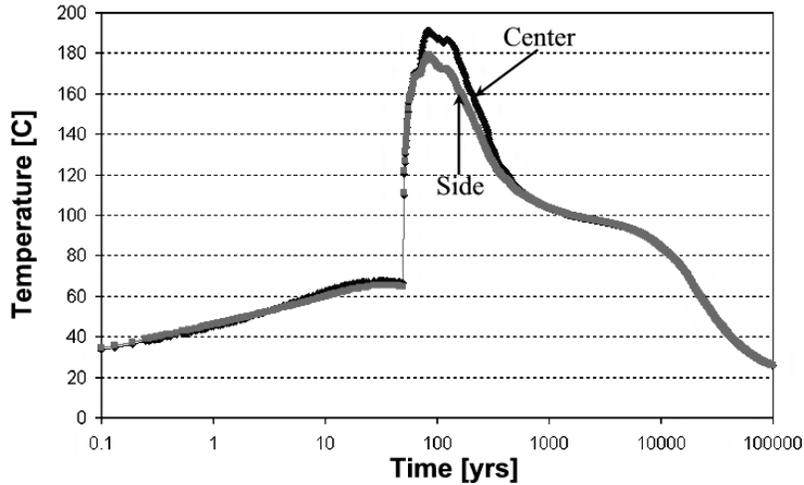
(a) Waste package temperature vs. time for Case 3.
