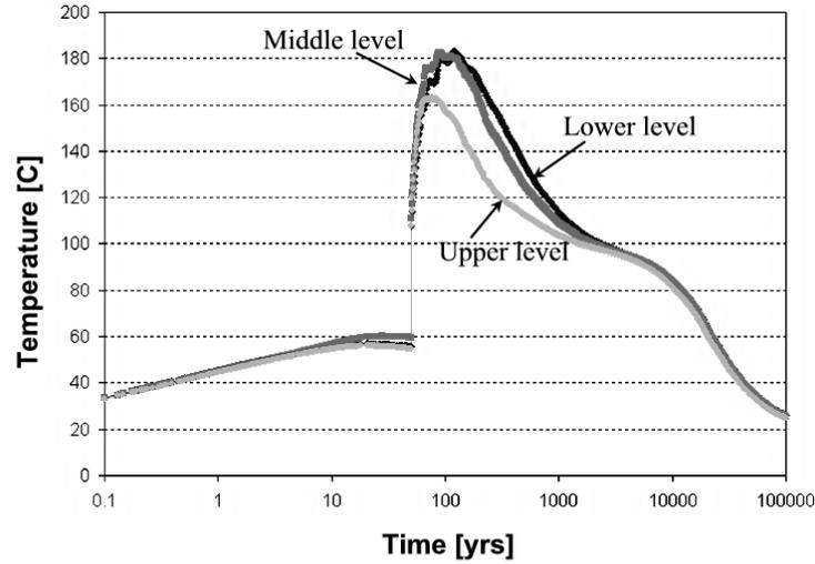
(a) Waste package temperature vs. time for Case 1.
