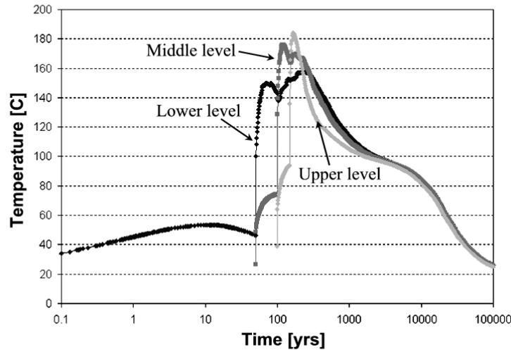
(b) Waste package temperature vs. time for Case 2.
