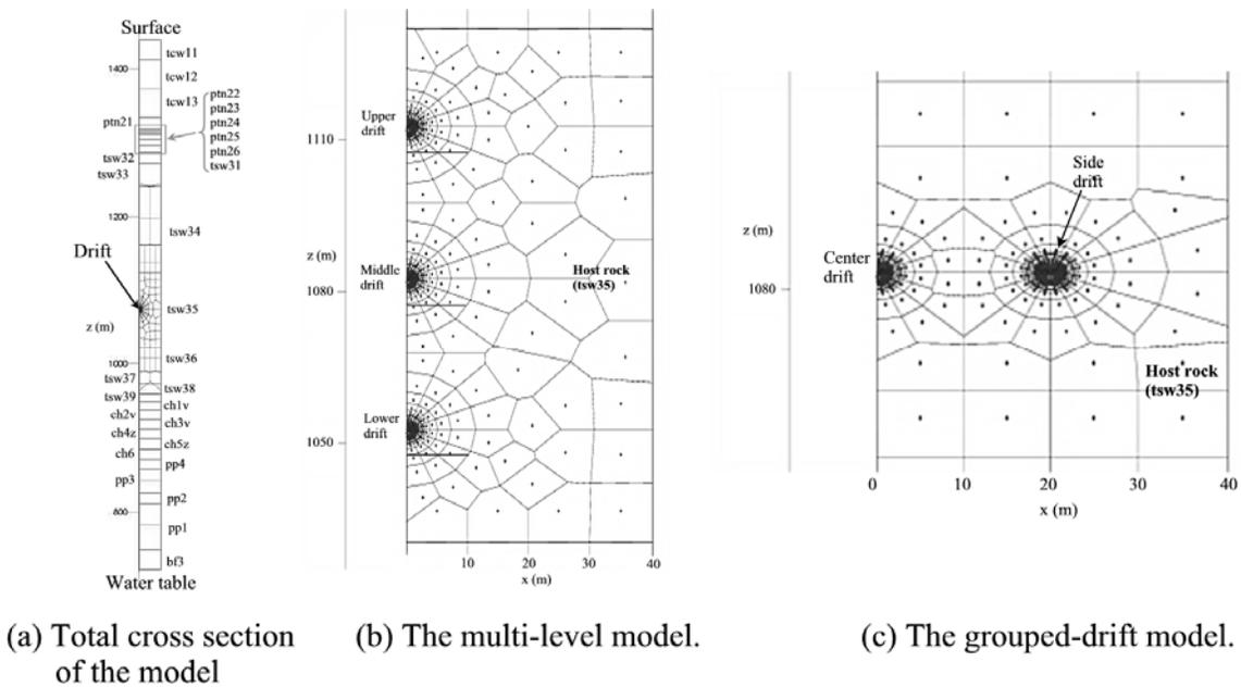
**Fig. 2. Description of the model for simulating thermal and hydrological response to the alternative repository designs.**
