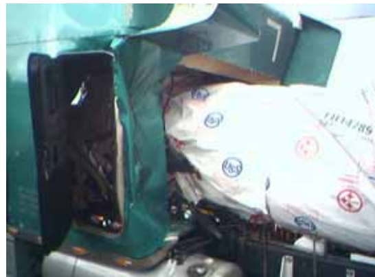
Figure 2. Steel from the trailer shifted into the driver's compartment.
