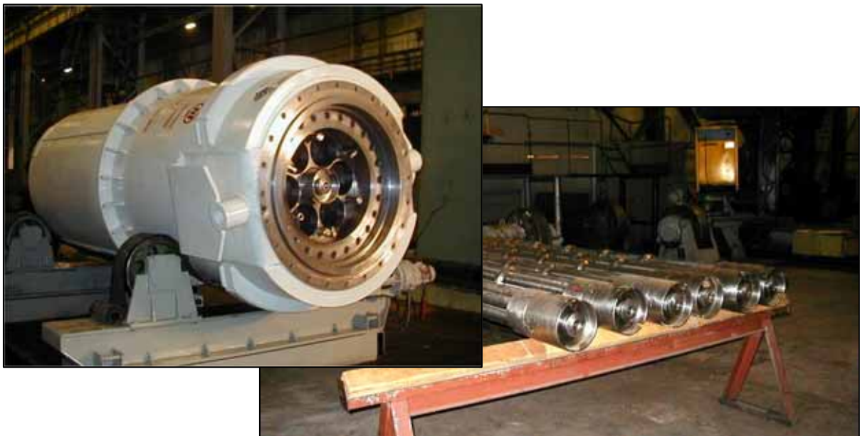
Fig. 2. TUK 108/1 Spent Fuel Cask and canisters for naval submarine fuel assemblies from decommissioned nuclear submarines
