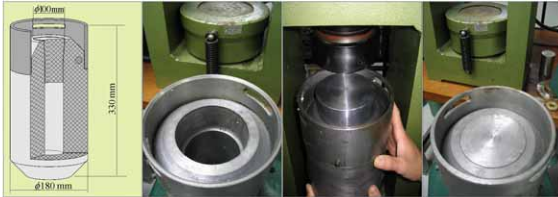
Fig. 2. Disposal package: a) cut view with dimensions; b) top view without the stopper; c) just before being sealed in a hydraulic press; d) a smooth top surface is left after stopper is inserted.
