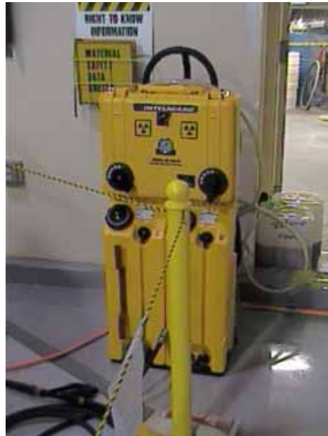
Figure 3. Foam generator/applicator for adding chemicals as a foam to the surfaces
