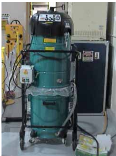
Figure 2. Wet/Dry HEPA vacuum for removal/collection of applied chemicals
