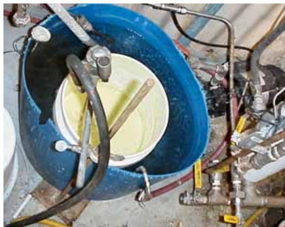
Fig. 20. Slurry container with agitator in heated bath.
