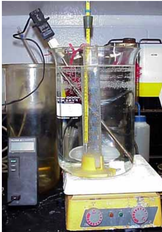
Fig. 13. Settling velocity test apparatus.
