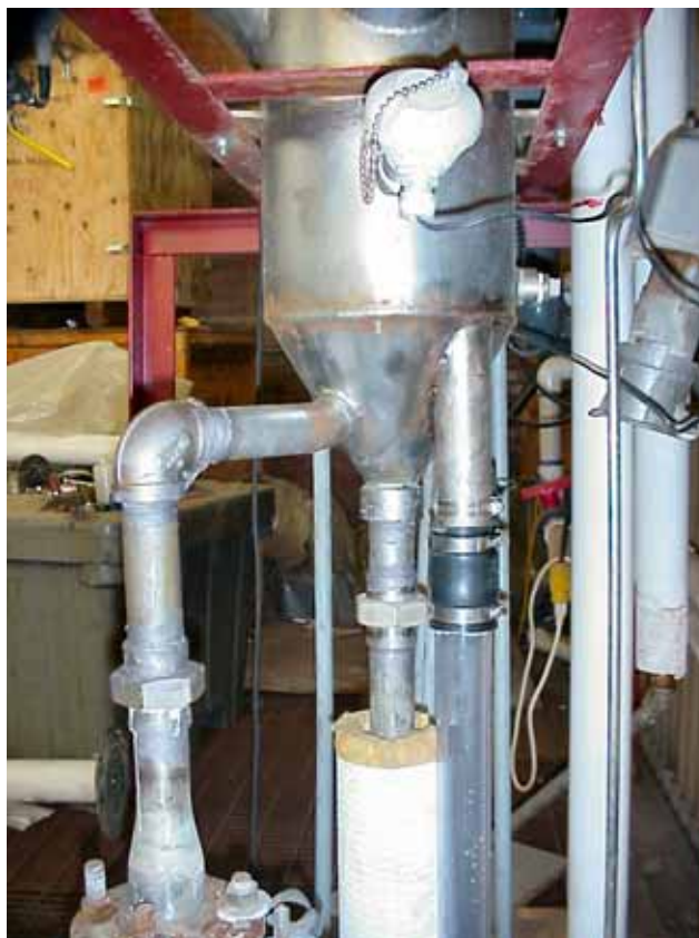
Fig. 16. DTE crystallizer with new elutriation leg.
