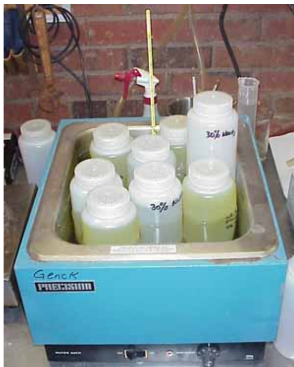
Fig. 19. Heated water bath for samples and wash.
