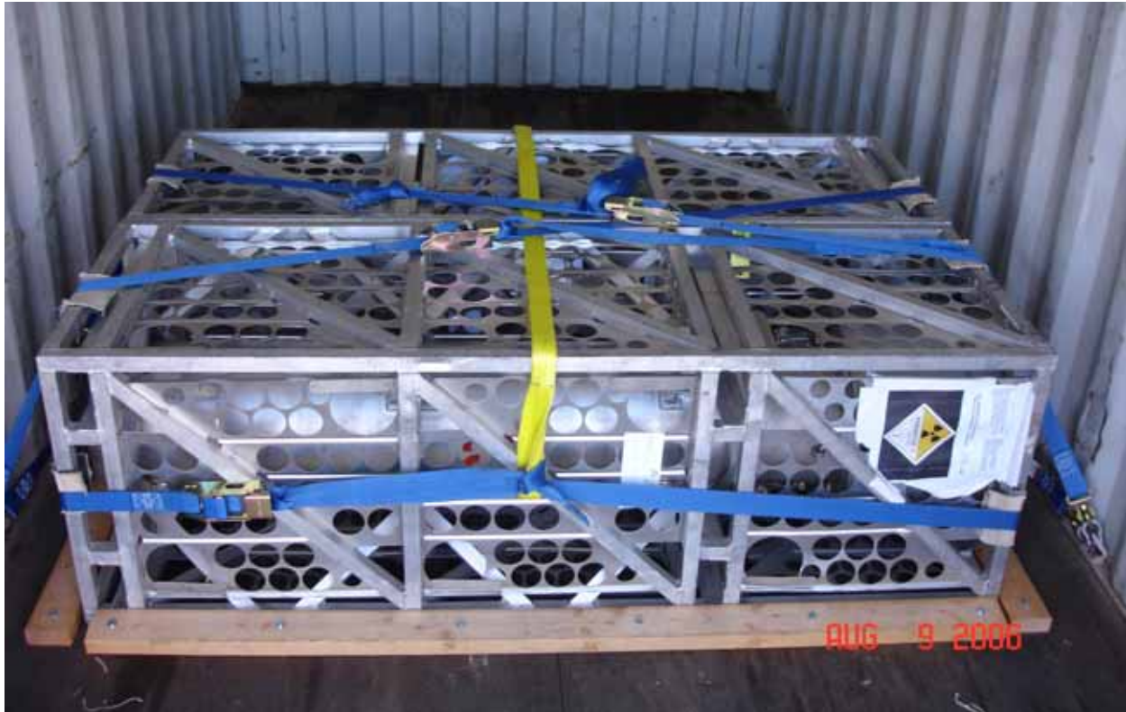
Figure 2. FUTURIX-FTA tie down configuration
