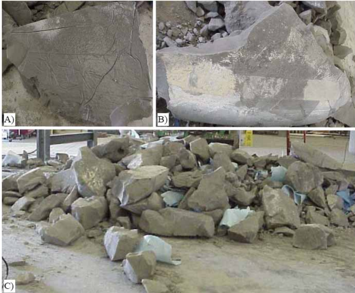
Figure 4: Pictures of the grout during breakup. A) Typical condition B) Edge of the tank. C) Overall after breakup
