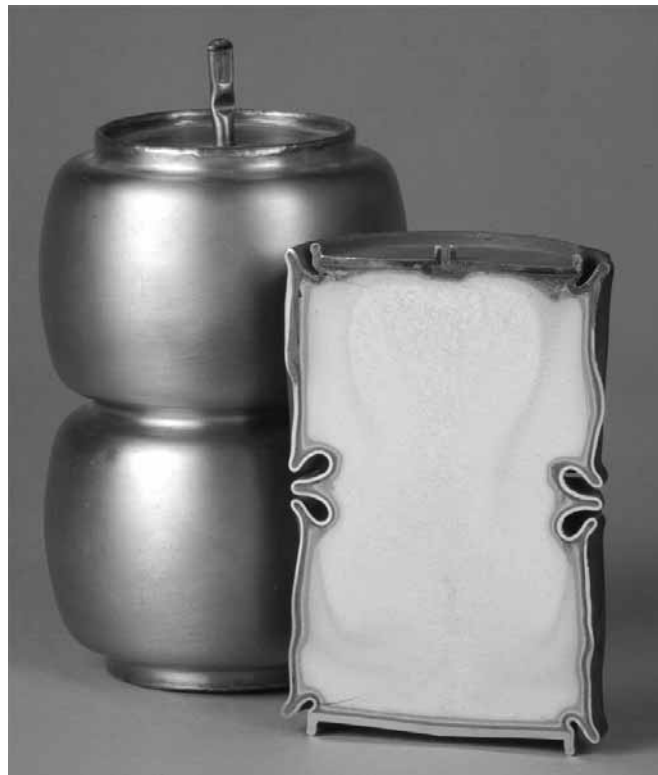
Fig 1 Example of HIPped ceramic product capable of being tailored for storage in a Magnox Pu can. (Illustration courtesy of ANSTO)
