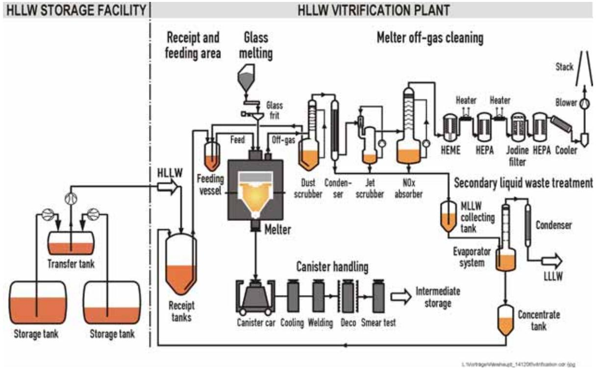
Fig. 1: Simplified diagram of the VEK vitrification process including the HLLW storage facility
