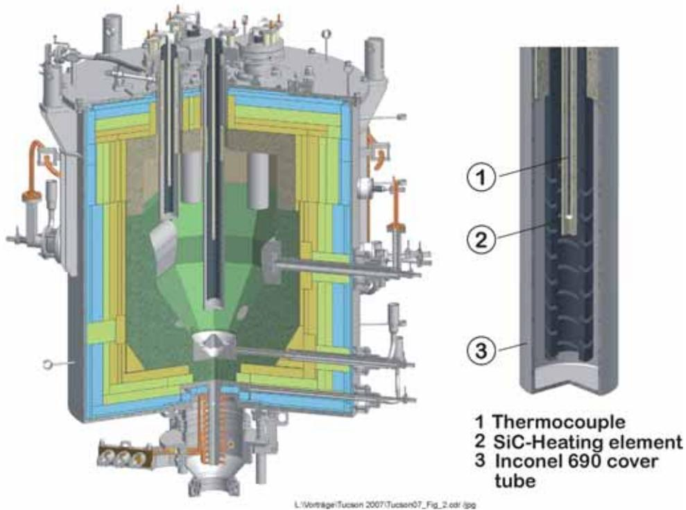
**Fig. 2:** Heating up of the internal melter structure by an external heat source (five SiC-heating elements encased in INCONEL 690 protection tubes including a thermocouple)
