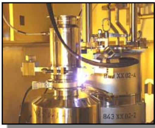
**Figure 4:** Demonstration of the canister lid welding in the canister handling cell of VEK. The chemical composition of the HLLW simulant will be as similar as possible to that of the radioactive HLLW. Radioactive samples have recently been taken from the HLLW storage tanks and analysed. Only
