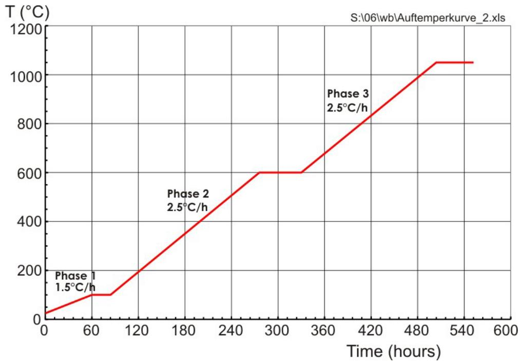
**Fig. 3:** Temperature vs. time curve for heating up of the inner melter structure
