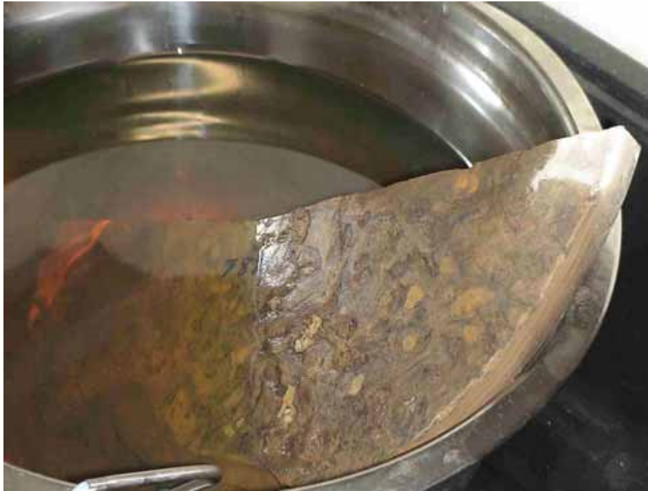
Figure 1: Waxfix permeation and wicking action in shale rock
