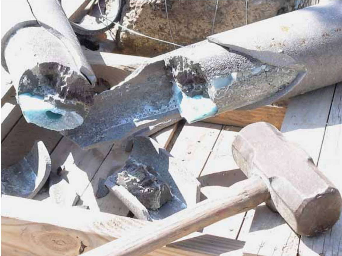
Figure 4: Pipe 1, Dry bentonite surrogate with cement grout cap, broken with hammer
