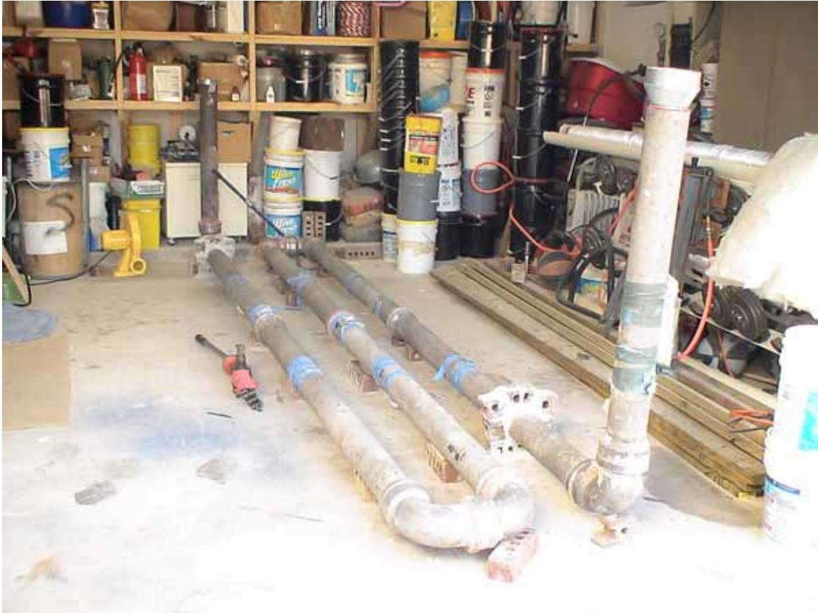
Figure 2: Pipe test loop after wax treatment and removal of soil
