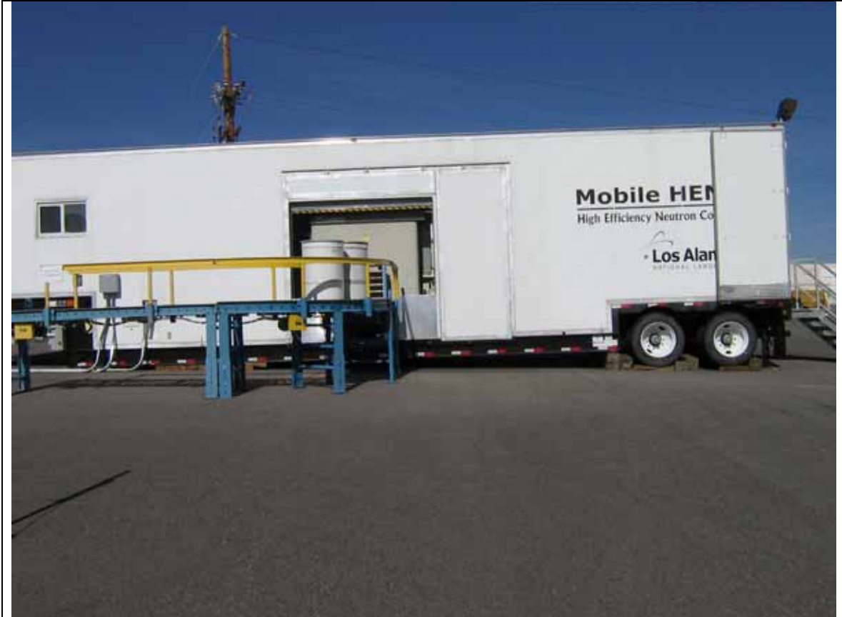
Figure 3: High efficiency neutron counter at Los Alamos National Laboratory (HENC#2).
