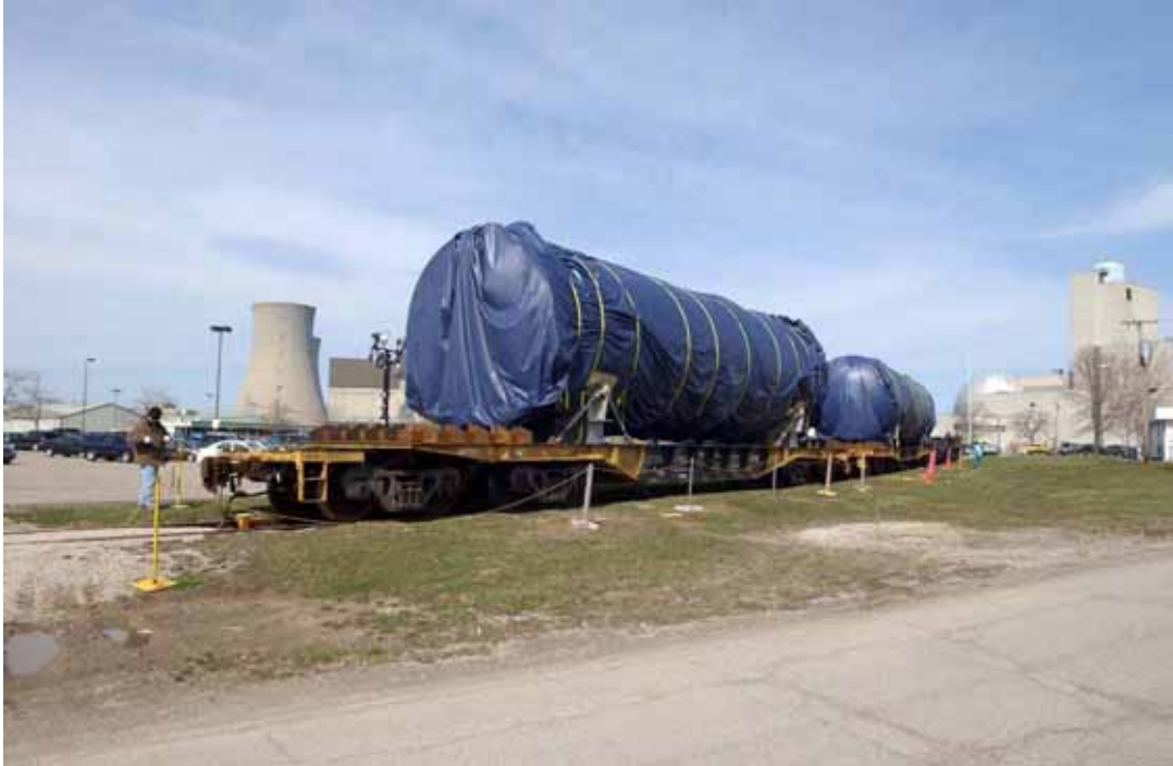
Figure 1: Fermi Main Steam Reheater halves on railcars
