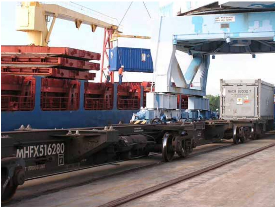
Figure 2: NAC Intermodal spent fuel containers loaded on MHF-LS railcars
