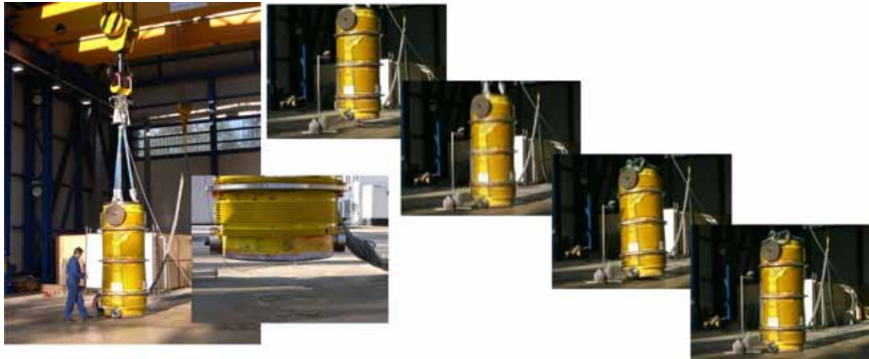
Fig. 2. 0.3 m vertical drop test at BAM with CASTOR ® HAW/TB2 onto the 2,600 Mg IAEA target
