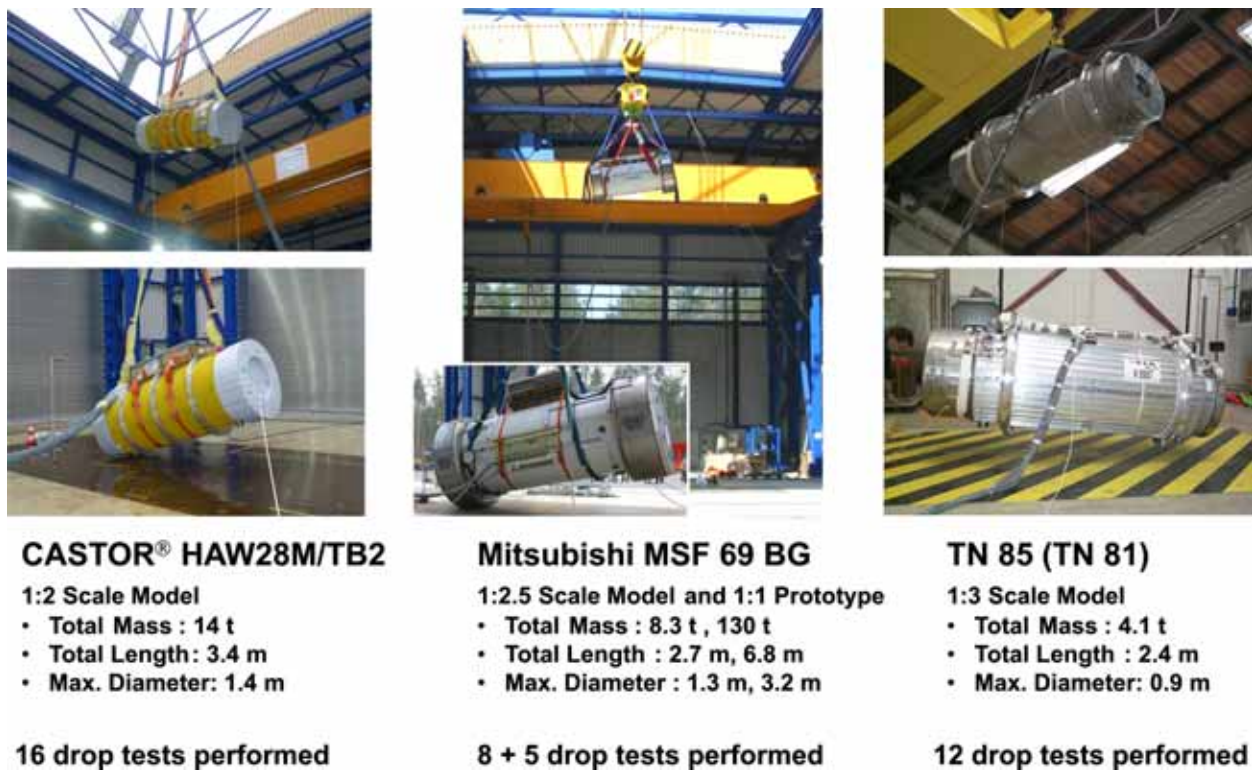
Fig. 1. BAM drop test series in 2004 - 2006 with new cask designs
