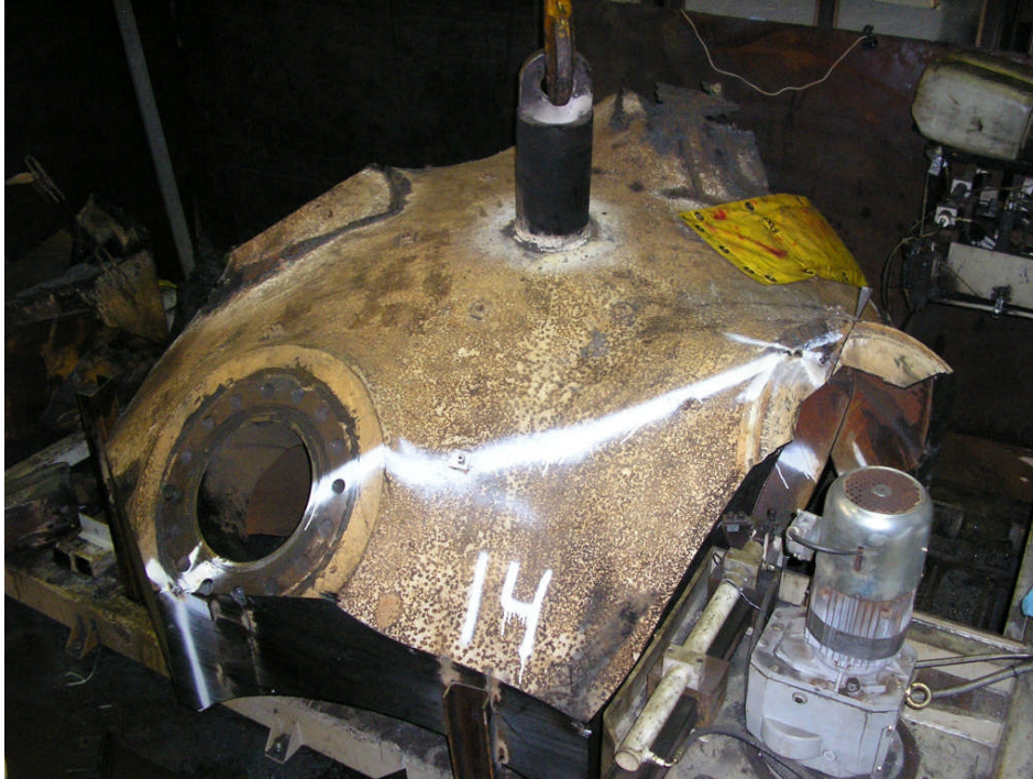
Fig. 4 Water chambers in the band saw.
