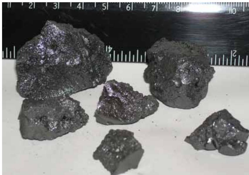
**Fig.3. Samples of melted DUO<sub>2</sub>.**
