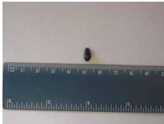
**Fig.5.  $\text{DUO}_2$  granule produced by draining the melt through hole in graphite crucible bottom.**
