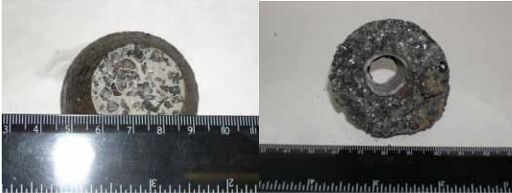
**Fig. 6. Samples of cast cermet  $\text{DUO}_2$ –stainless steel.**
