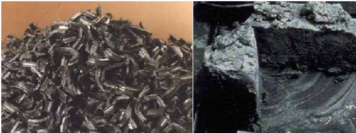
Figure 1 Fresh Magnox swarf and corroded Magnox sludge
