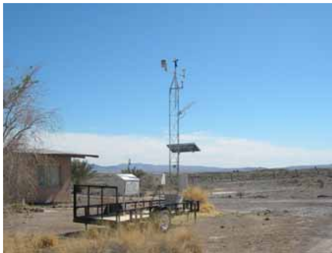
Figure 5. A CEMP mobile trailer-mounted monitoring station near Tecopa, California.
