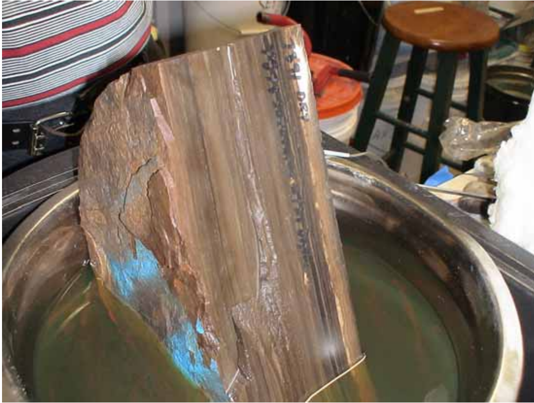
Figure 1: After 24 hours in Waxfix, capillary action has saturated this rock
