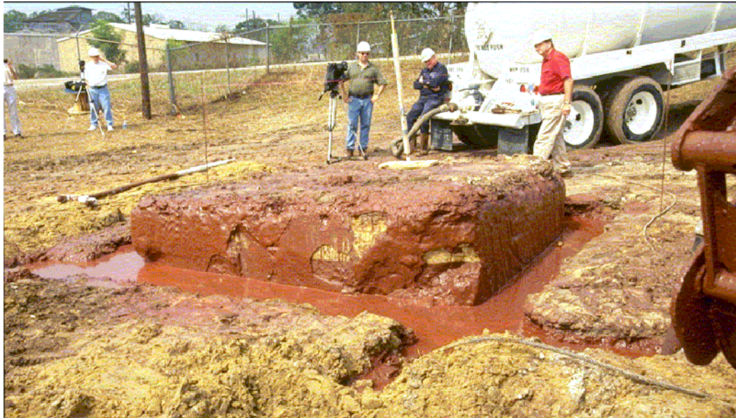
Figure 3: First Field Demonstration Floating a Block of Earth Severed With Steel Cable
