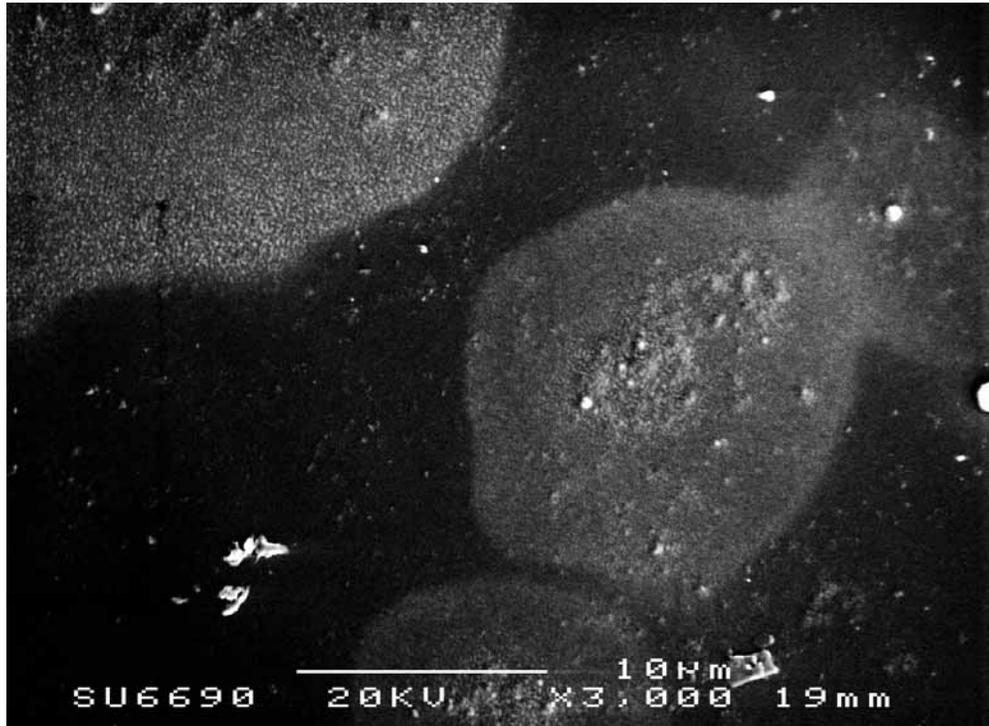
**Fig.2. British Magnox-waste glass secondary electron image (JEOL 6400 scanning electron microscope operating at 20kV).**
