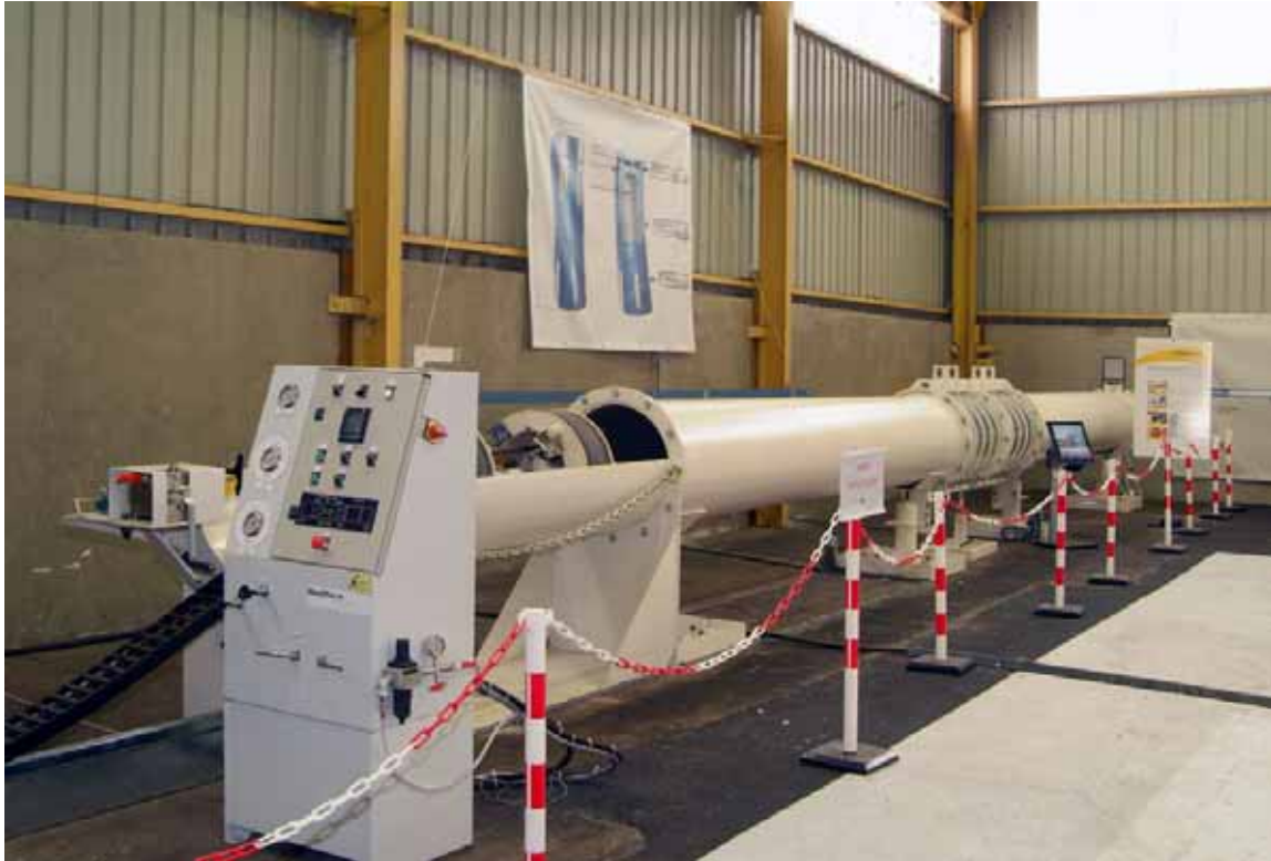
Fig. 4. General view of the test bench, also showing the Prototype Pushing Robot and the Control Panel
