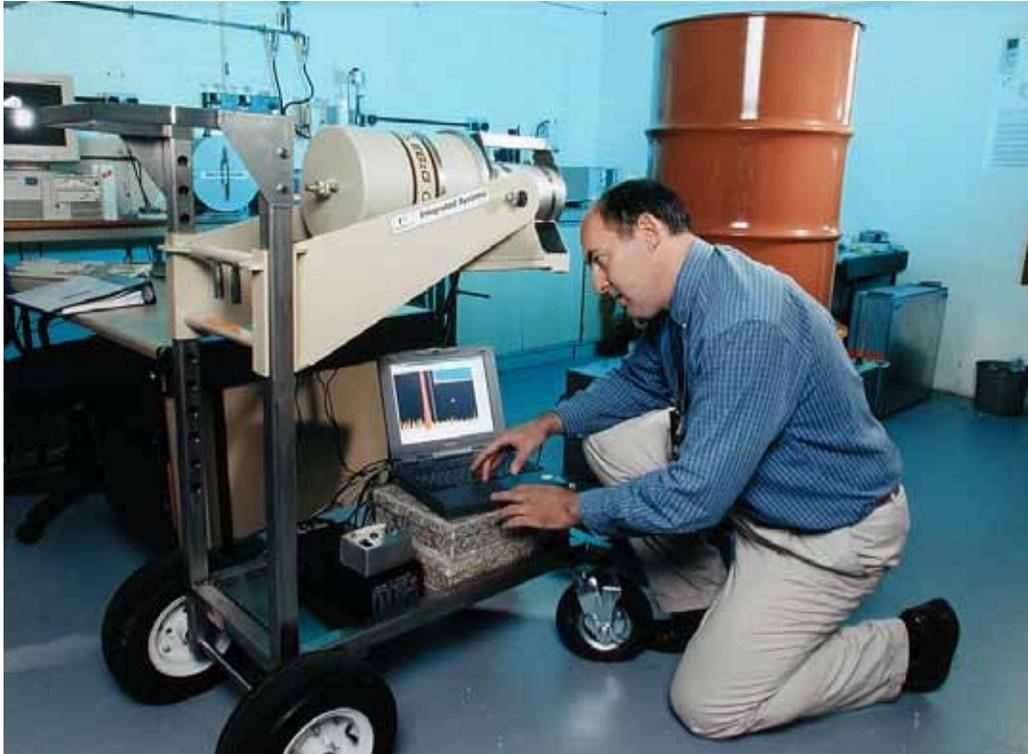
**Figure 1** HRGS monitoring a waste drum on a turntable
