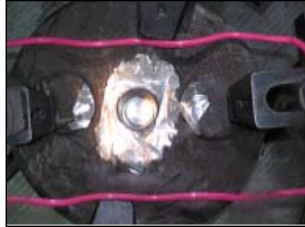
Fig. 4. Reflection of the stuck 6.6 mCi Ra-226 after drilling
