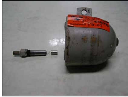
Fig. 2. Ra-226 cylindrical type fixed with iron spring
