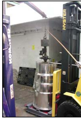
Fig. 3. Ra-226 loading in lead shield
