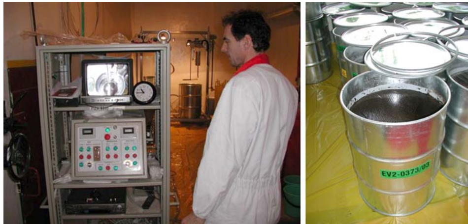
Fig. 4. Solidification of sludges from the "TR" tank into the SIAL matrix by the remote operated device and the solidified product in drums
