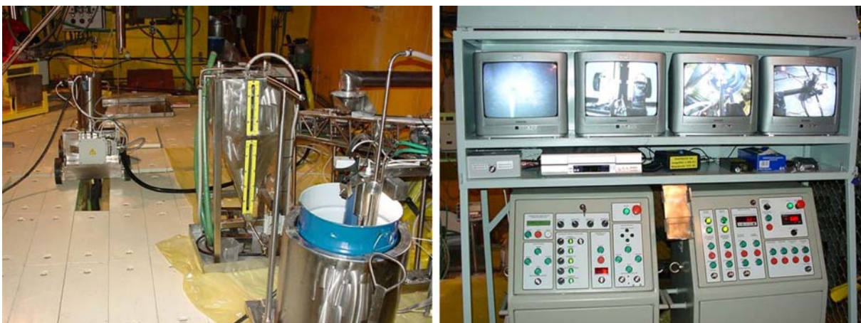
Fig. 2. Devices and control board used for the remote operated works in the fuel storage pool
