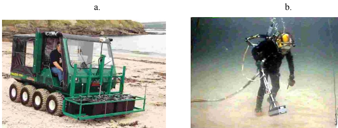
Fig. 2. Monitoring Particle location a) using the Groundhog™ system at Sandside and b) divers off the coast at Dounreay.
