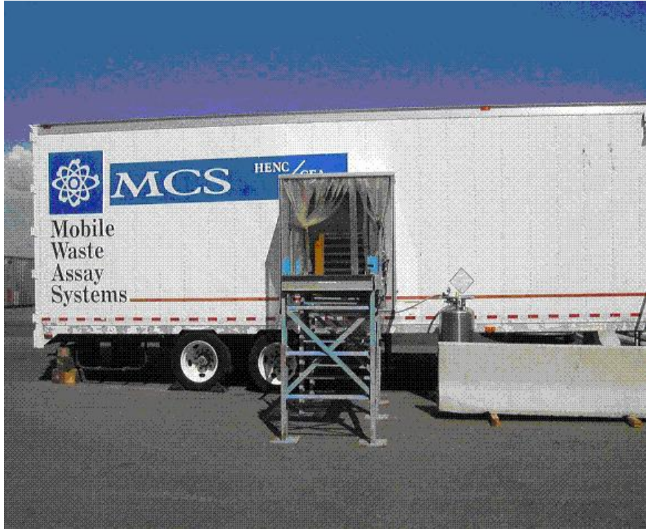
Fig. 1. MCS HENC trailer showing conveyer assembly
