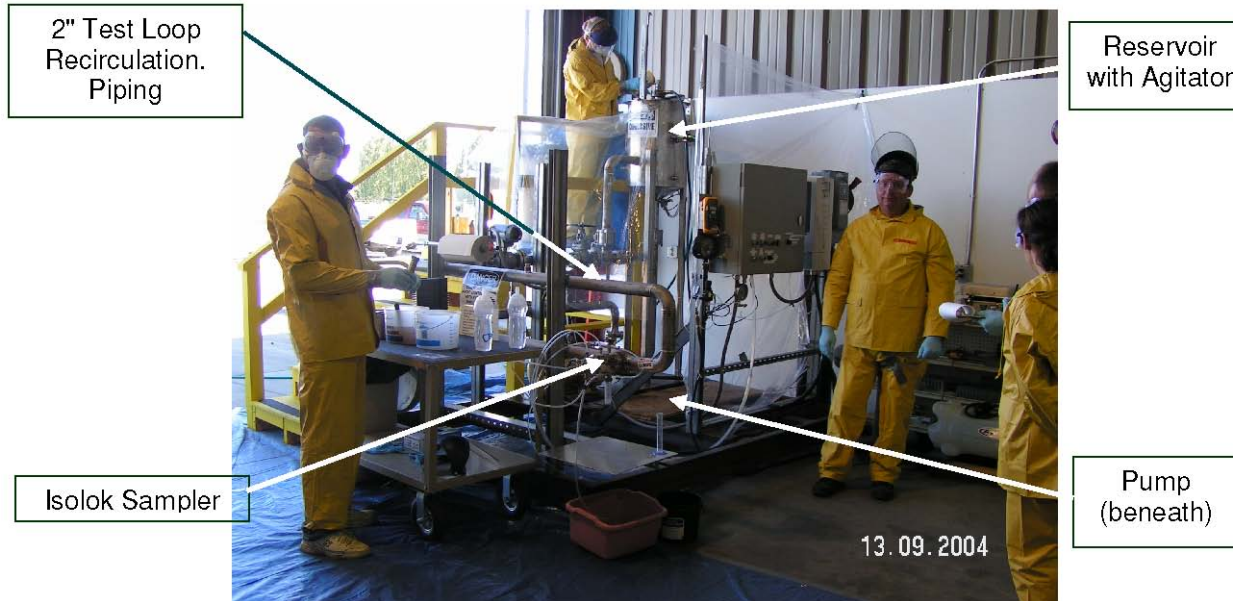
Fig. 4. Sampling device performance test loop
