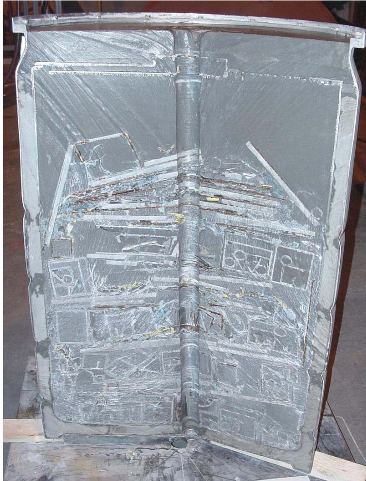
Fig. 1. Sectioned drum showing inactive encapsulated waste
