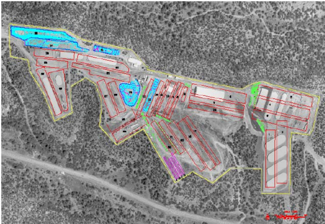
(Blue outlines currently active units; red outlines formerly used units; green outlines shaft fields; purple outlines trenches; and white structures are fabric domes.)
