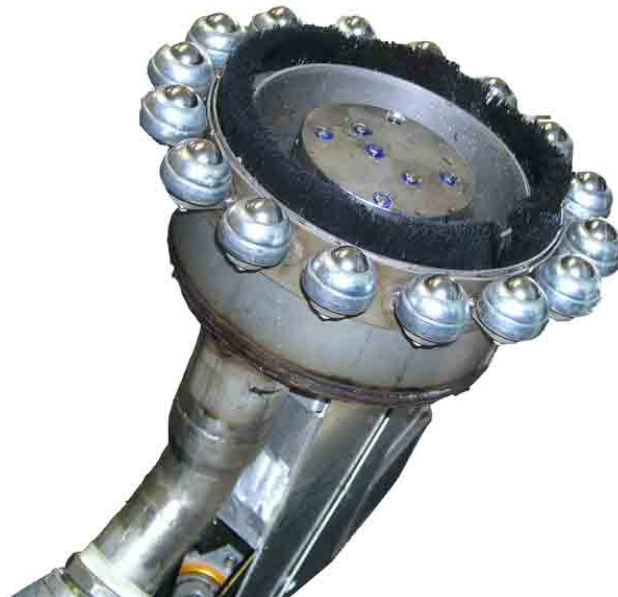
Fig. 4. Hydromilling nozzles mounted inside vacuum recovery shroud
