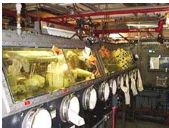
Plutonium Finishing Plant glovebox to be removed
