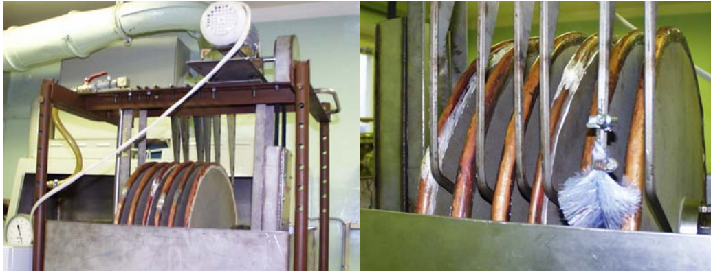
Fig. 6. Overview of “Augean” disc vacuum filter ( S_{\text{filtering area}}=2 \text{ m}^2 )
