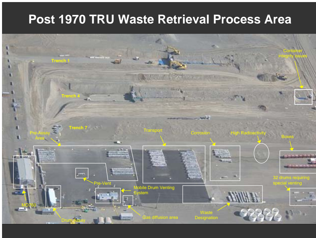
Fig. 3. Retrieval process area, indicating process operations and staging areas.
