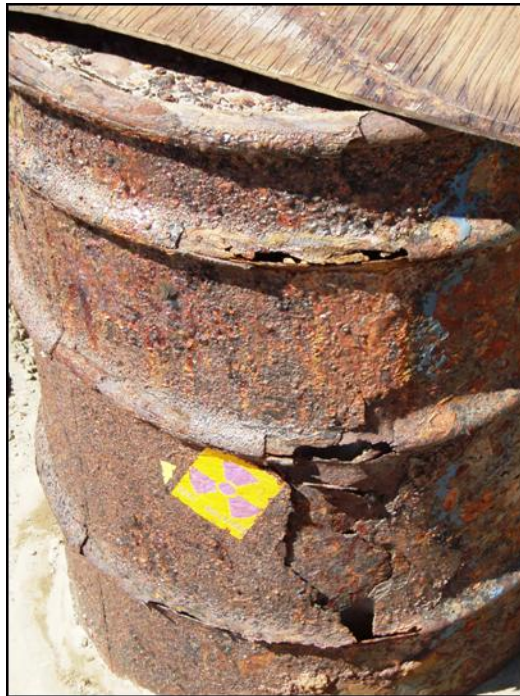
Fig. 2. Severely corroded drum, requires overpacking
