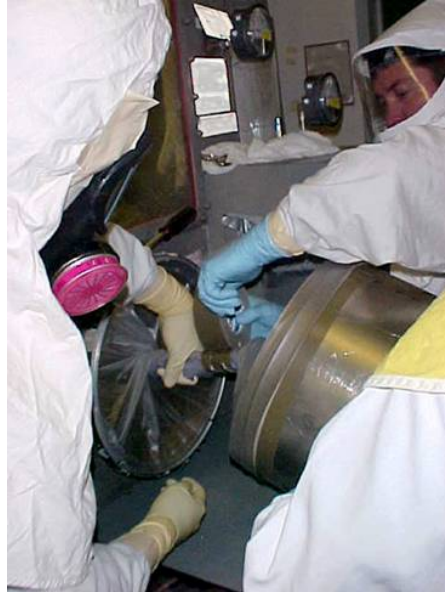
Fig. 1. The rigid port bag being used to remove contaminated glovebox equipment.
