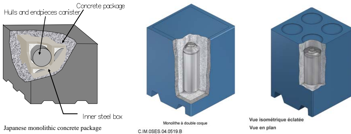
Fig. 2. RWMC and Andra package designs for long-term performance: application to hulls and end pieces
