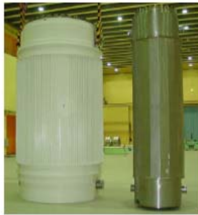
Fig. 1. TN TM 24BH and TN TM 9/4 metal casks in ZWILAG storage hall
