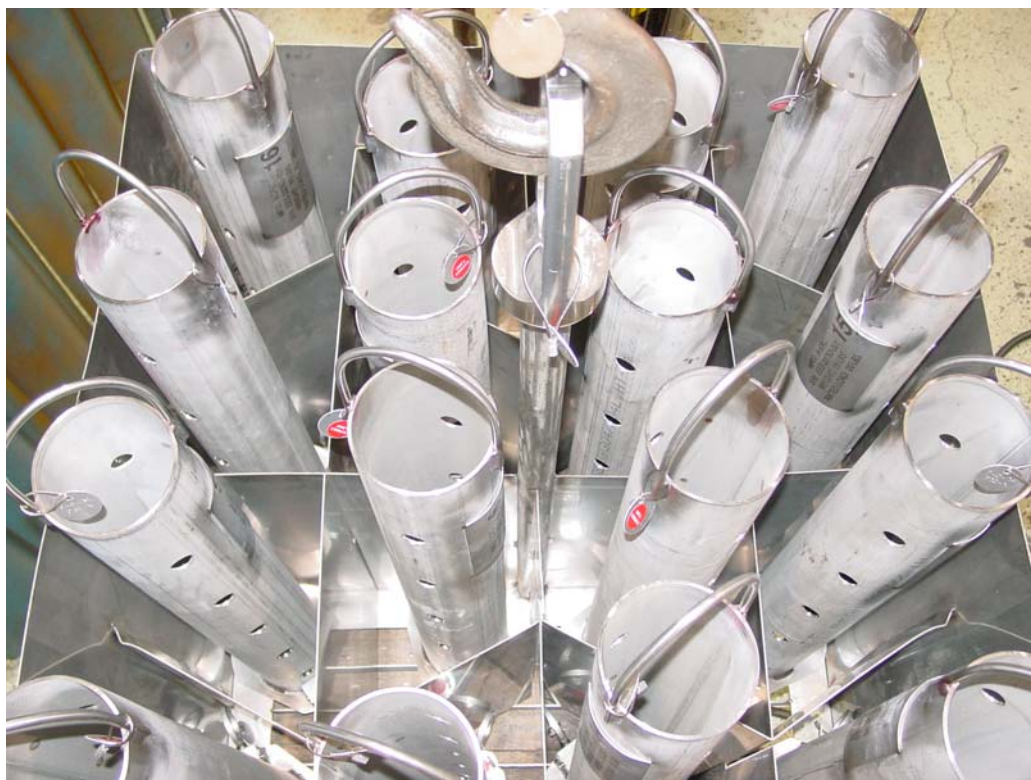
Fig. 2. Sixteen beaker magazines (empty) loaded into magazine rack
