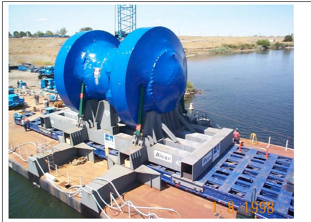
Fig. 3. Final reactor barge transportation design
