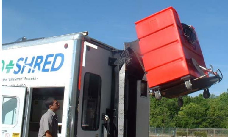
Fig. 4. A plastic cart containing surrogate medical waste is lifted and dumped into the shredder hopper during a treatment capability demonstration
