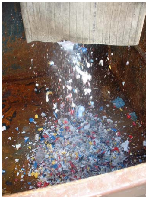
Fig. 7. Typical appearance of shredded and disinfected medical waste. This photo shows shredded and treated surrogate medical waste materials, consisting of non-contaminated paper materials, plastic materials (plastic drinking cups), cloth materials (shop rags), and glass materials (glass drinking cups)
