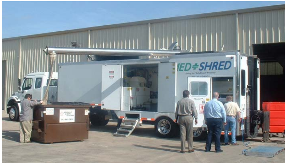
Fig. 2. Typical truck-mounted Med-Shred medical waste treatment system seen during a treatment capability demonstration
