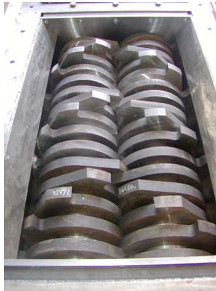
Fig. 5. A top view looking inside a low-speed, high torque shredder. Teeth on counter-rotating discs bite into and pull material between the two shafts, cutting the material into smaller pieces
