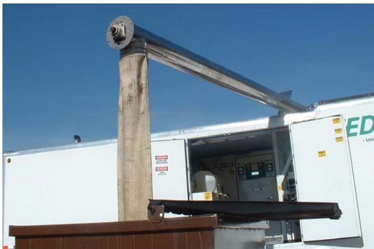
Fig. 6. The boom is used to transport treated waste from the processor to a hospital compactor or other container for the treated waste
