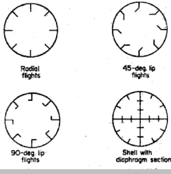
Fig. 3. Design of internal flights of Rotary Calciner
