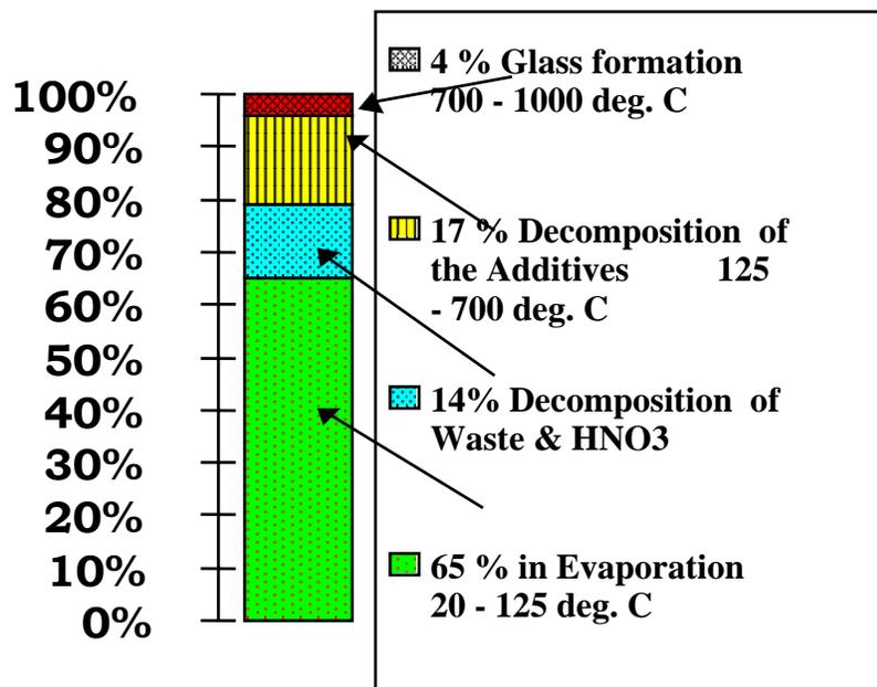
Fig. 1. Thermal energy in volume reduction processes
