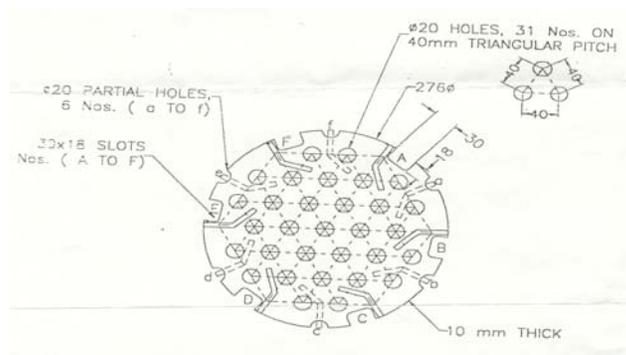
Fig 2. Design of central grid plates
